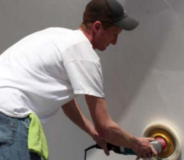
*Detailing the hull and deck make old fiberglass gleam.*
