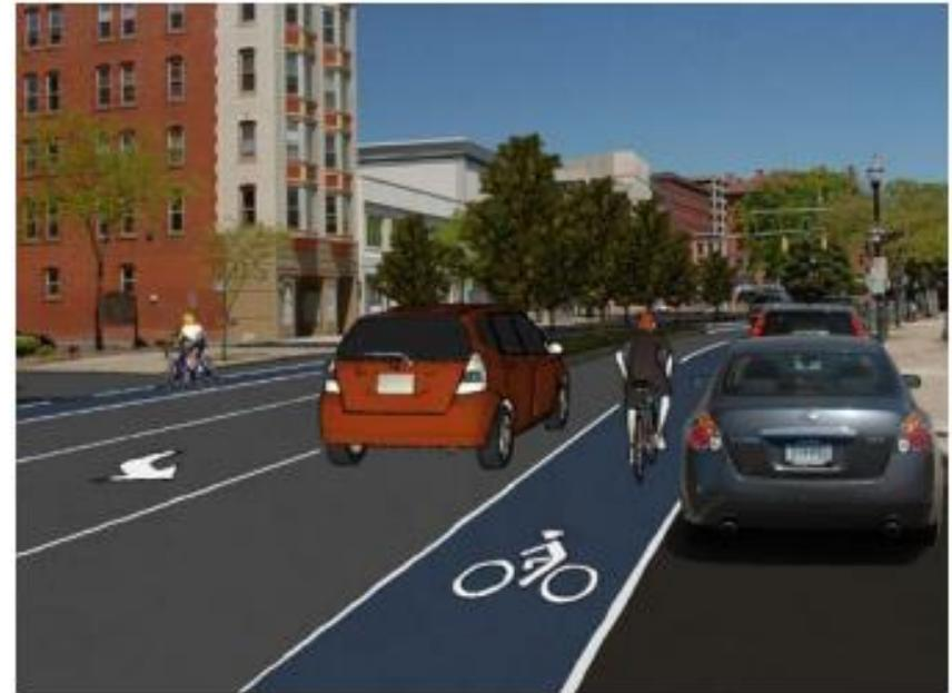
This "before and after" section of Main Street looking north illustrates how it could be reshaped with a road diet to be a Complete Street.
