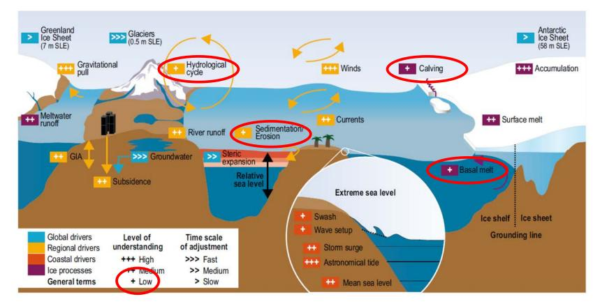
Figure 4.4 | A schematic illustration of the climate and non-climate driven processes that can influence global, regional (green colours), relative and extreme sea level (ESL) events (red colours) along coasts. Major ice processes are shown in purple and general terms in black. SLE stands for Sea Level Equivalent and reflects the increase in GMSL if the mentioned ice mass is melted completely and added to the ocean.
