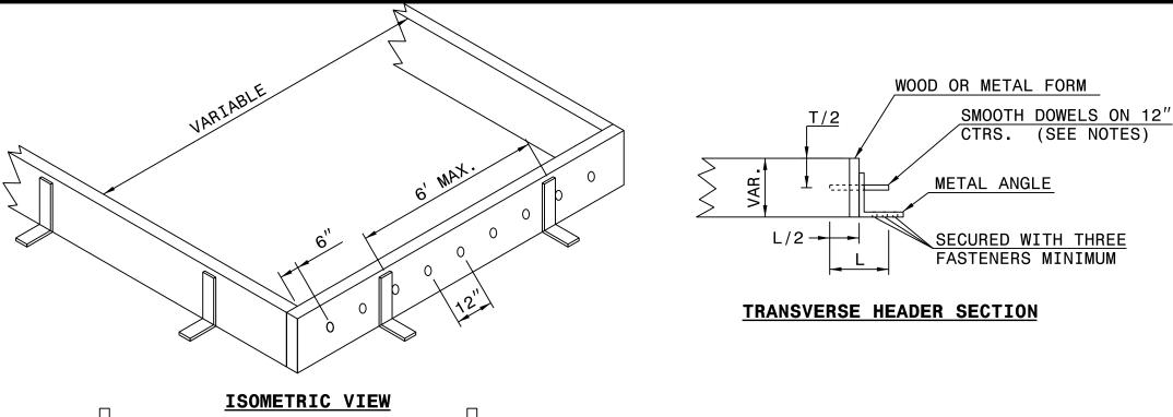
000 . . . **VARIABLE** NOTE: UPON COMPLETION OF FINAL SLAB, REMOVE METAL OR 000 WOODEN FORM 000 DOWEL DIA. +  $\frac{1}{16}$ " 12" 6" SECURED WITH THREE FASTENERS MINIMUM 6' MAX.
