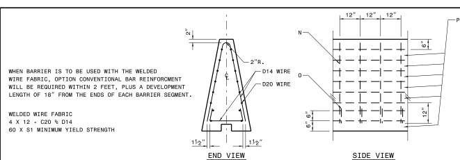
WELDED WIRE FABRIC OPTIONAL REINFORCING
