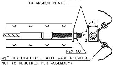
$^3/8"$  THICK END PLATE WITH  $^1/_6"$  DIA. HOLE CENTERED IN PLATE. END PLATE TO BE WELDED
