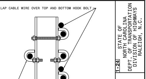
THE CENTER POST IN THE INTERMEDIATE ANCHORAGE SECTION WILL HAVE CABLE WIRE ON BOTH SIDES OF THE MIDDLE STRAND REQUIRING THE USE OF TWO 134" HOOK BOLTS FOR THIS APPLICATION.
