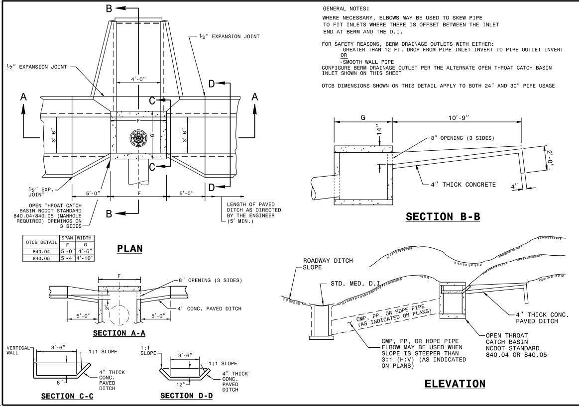
**OUTLET** INLET PIPE FOR 30,, BASIN DRAINAGE DRAWING AND CATCH 24" STANDARD OPTION BERM **THROAT** ROADWAY FOR ALTERNATE WITH OPEN
