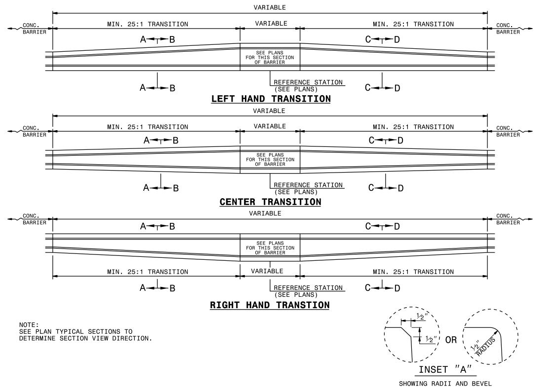
BARRIER ASSEMBLY FOR TRANSITION STANDARD DRAWING OVERHEAD MEDIAN 0F LOCATION ROADWAY CONCRETE
