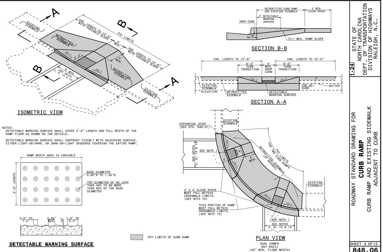
SIDEWALK DRAWING ISTING **RAMP** STANDARD EX CURB AND RAMP ROADWAY CURB
