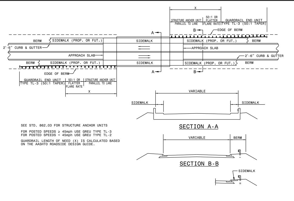
STANDARD GUARDRAIL PLACEMENT AT BRIDGES WITH 2'-6" CONCRETE CURB AND GUTTER
