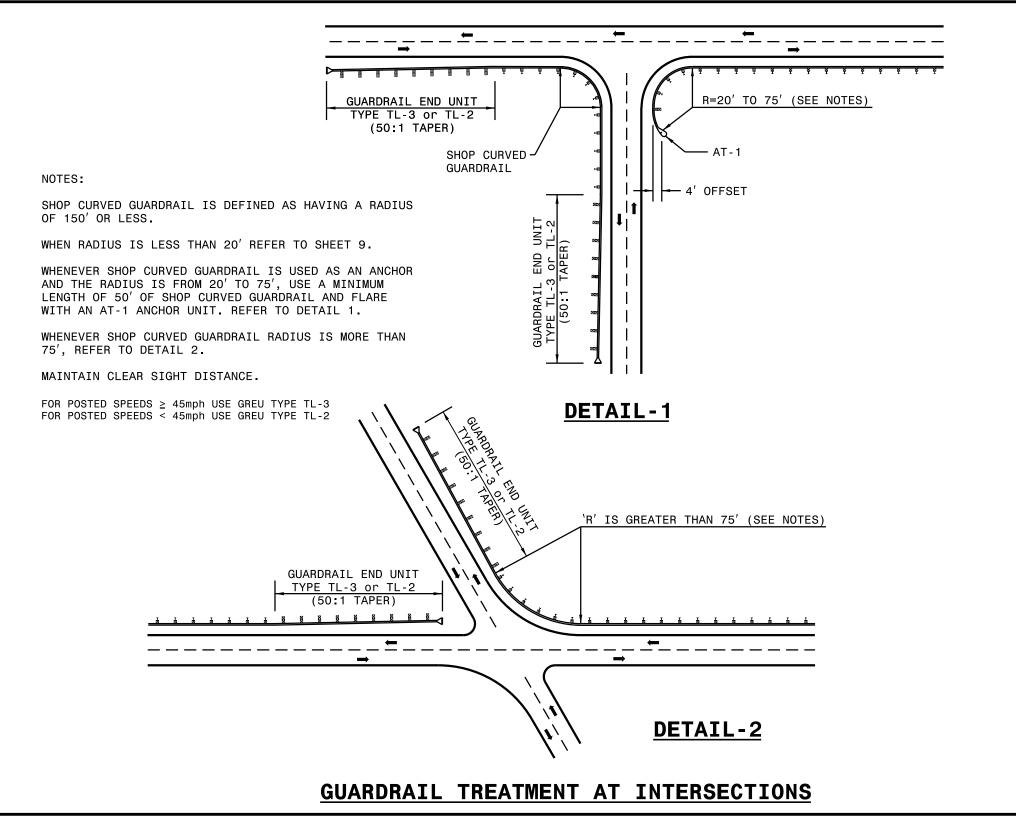
ROADWAY STANDARD DRAWING FOR GUARDRAIL PLACEMENT
