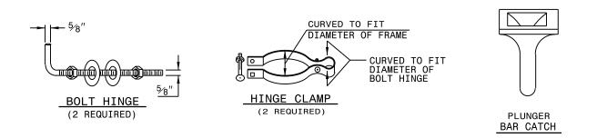
USE LATCH DEVICE APPROVED BY THE ENGINEER. HINGE ASSEMBLY, AS DETAILED, IS SUGGESTED. SUBSTITUTION MAY BE MADE SUBJECT TO APPROVAL BY THE ENGINEER. USE 13/8" DIAMETER GALVANIZED STEEL PIPE GATE FRAME EXCEPT AS SHOWN HERE.
