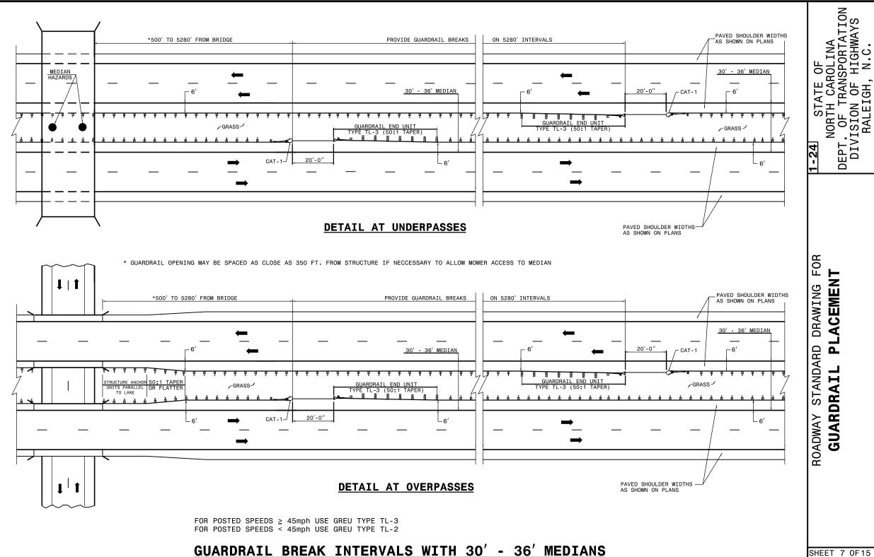
FOR **PLACEMENT** DRAWING STANDARD GUARDRAIL ROADWAY
