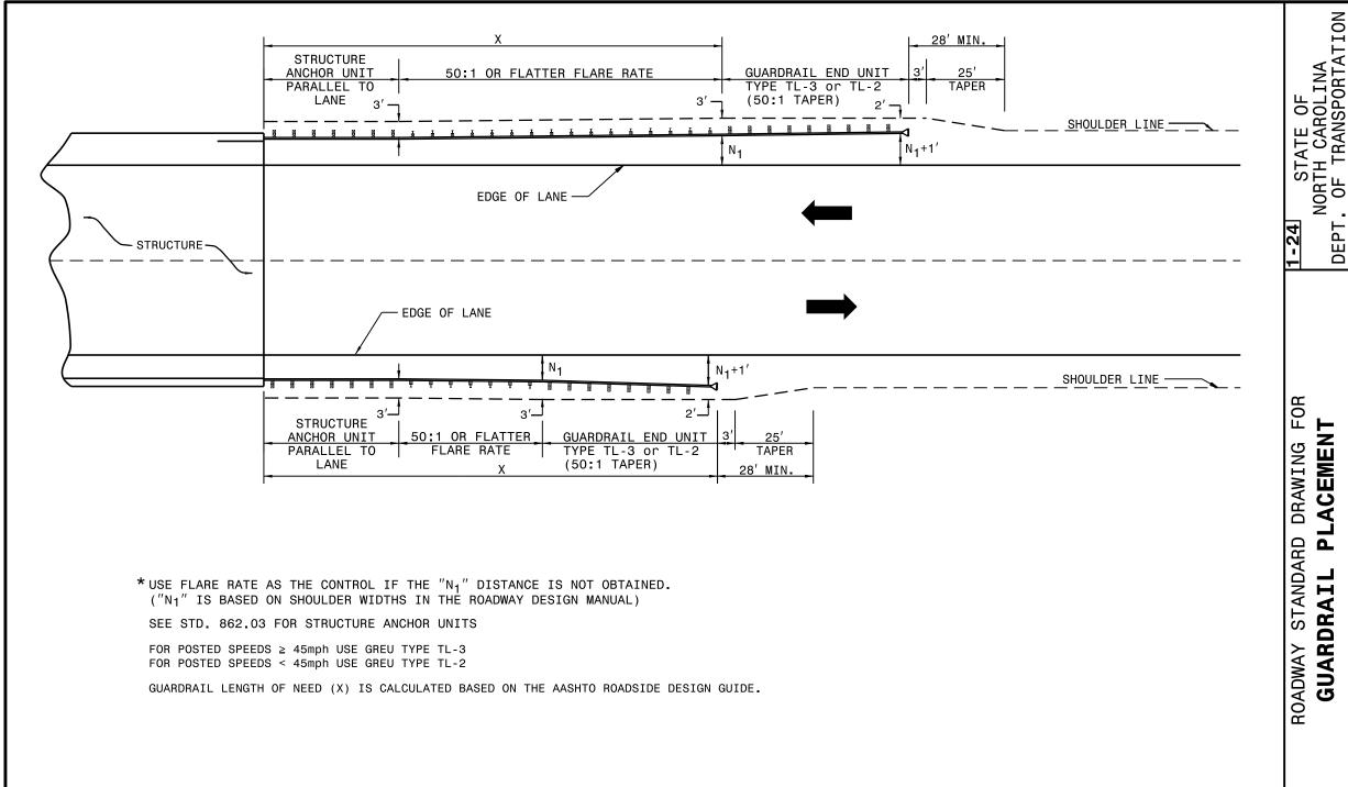
LENGTHS AND OFFSETS FOR PROPOSED GUARDRAIL AT TWO LANE - TWO WAY LOCATIONS
