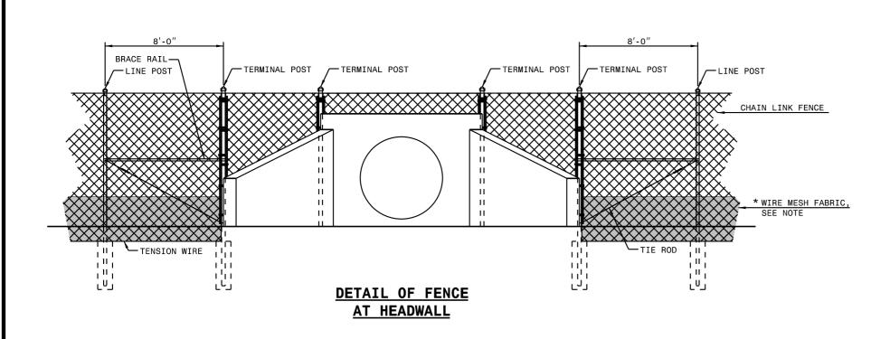
ROADWAY STANDARD DRAWING FOR WILDLIFE FENCE WITH CHAIN LINK
