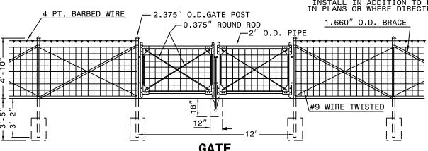
USE LATCH DEVICE APPROVED BY THE ENGINEER. HINGE ASSEMBLY, AS DETAILED, IS SUGGESTED. SUBSTITUTION MAY BE MADE SUBJECT TO THE APPROVAL OF THE ENGINEER.
