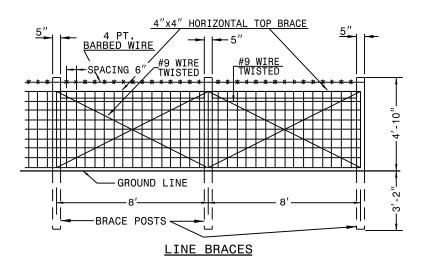
(MAXIMUM SPACING 324') PLACE THE BRACE WIRE AROUND THE POST. DRAW WIRE TAUT BY TWISTING BETWEEN EACH POST. THIS APPLIES TO ALL BRACE WIRES. NOTCH POSTS FOR BRACES. PLACE TWO GALVANIZED 12d OR THREE GALVANIZED 10d ON ALL BRACES AT EACH END.
