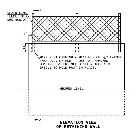
EMBED CHAIN LINK FENCE 11" INTO PROPOSED WALL IN A SLEEVE OR BLOCKOUT WITH EPOXY OR CONCRETE GROUT ANCHORING SYSTEM. PRE-MEASURE AND CENTER THE PROPOSED FENCE ON TOP OF WALL FOR POST SPACINGS. IF DRILLING THE HOLES FOR POSTS, USE A ROTARY DRILL TO DRILL HOLES IN THE CONCRETE. NO IMPACT DRILLS WILL BE ALLOWED, TO ELIMINATE ANY POSSIBILITY OF STRUCTURAL DAMAGES TO THE PROPOSED WALL.
