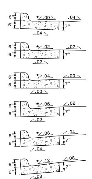
THE GUTTER SLOPE FOR 1'-6" CURB AND GUTTER SHALL MATCH THE SLOPE OF THE ADJOINING PAVEMENT.
