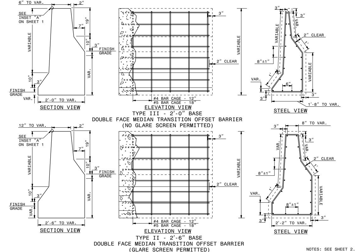
BARRIER ASSEMBLY TRANSITION STANDARD DRAWING OVERHEAD MEDIAN 0F LOCATION ROADWAY CONCRETE
