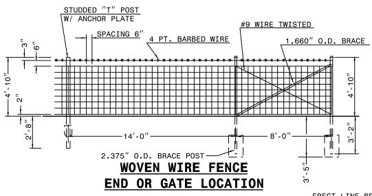
2.375" O.D. BRACE POST #9 WIRE 1.66" OD SPACING 6' 4 PT. BARBED WIRE
