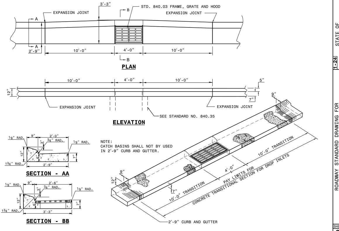
BEARING **GUTTER**) OP INLET CURB AND TRAFFIC GRATED DROP (FOR USE WITH 2'-9" CU FOR CURB MEDIAN
