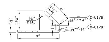
NOTE: SUBMIT ALTERNATE METHODS OF FABRICATING ANCHOR ANGLES FOR APPROVAL.
