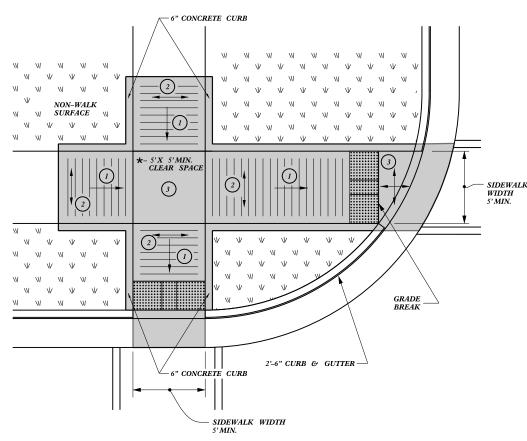
\* - WHERE CLEAR SPACE IS CONSTRAINED ON TWO OR MORE SIDES, THE CLEAR SPACE SHALL BE 4 MINIMUM X 5 MINIMUM, WITH 5 PROVIDED IN THE DIRECTION OF THE PEDESTRIAN STREET CROSSING.
