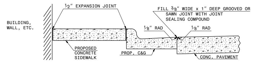
DETAILS SHOWING JOINTS IN CONCRETE SIDEWALK
