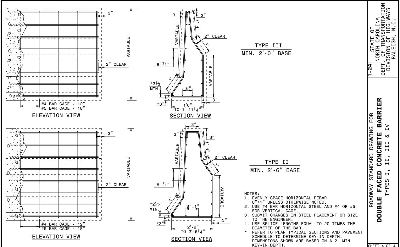
STEEL PLACEMENT FOR CAST-IN-PLACE OR SLIP-FORM CONCRETE BARRIER
