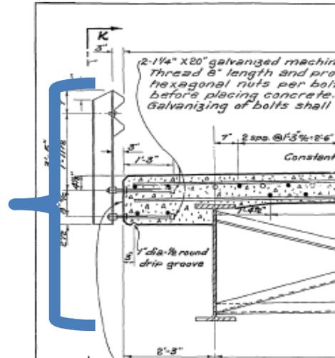
Figure 2 - Offset Distance in this example is not on the plans and needed field measured
