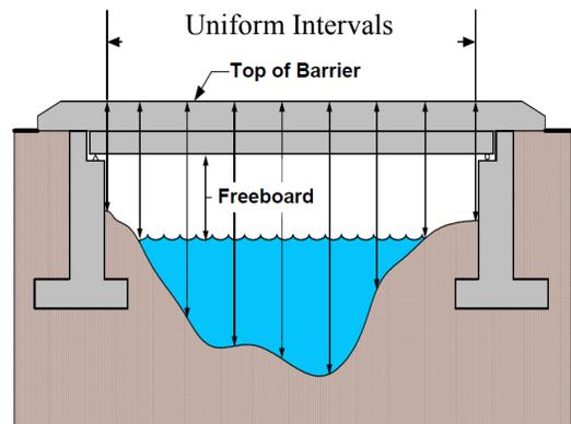
Figure 3 - Channel Cross Section Intervals (NHI)
