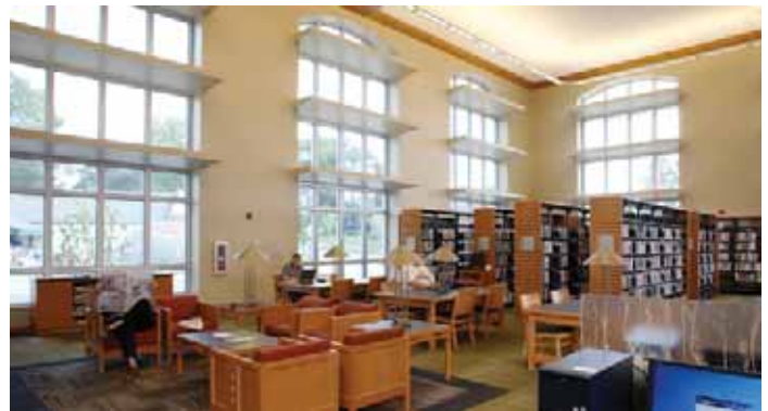
Light shelves help reduce energy costs
