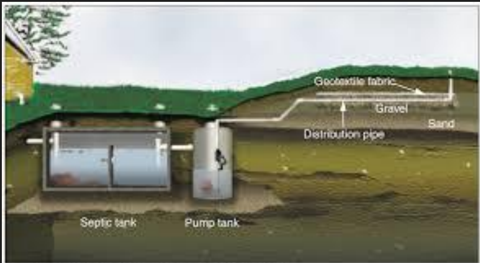
Figure 1: A mixed system for distributing treated waste water to the soil.
