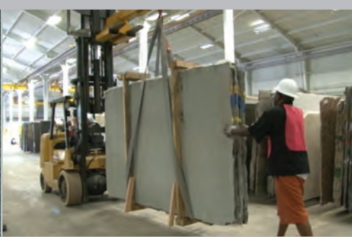
Moving slabs with forklift and spotter
