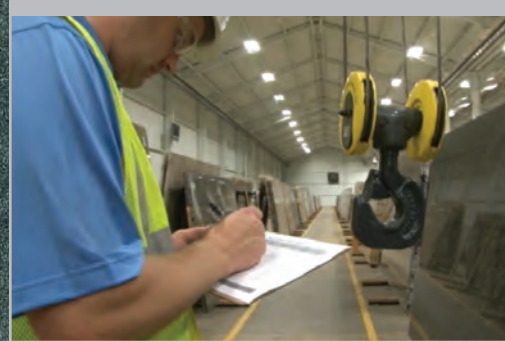
Worker with inspection checklist for hoist
