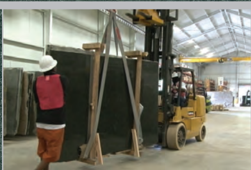
Stone slab moved by forklift
