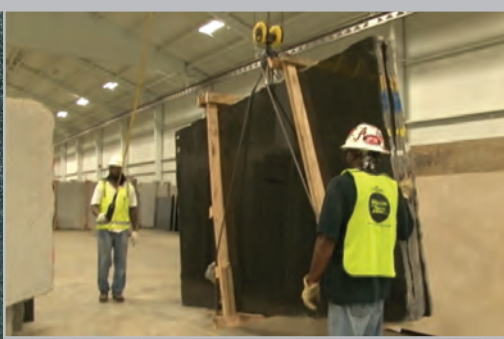
Moving a slab with an overhead crane
