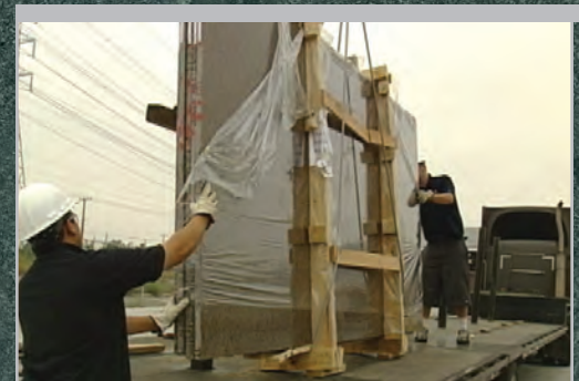
Bundles on flatbed without A-frame or poles
