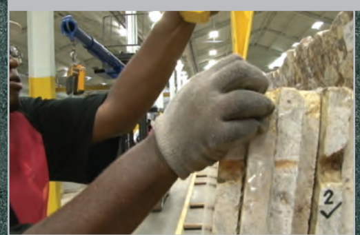
Worker wearing proper gloves while working with slab that has rough edges
