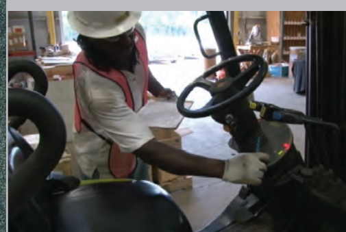
Inspection of driver's area of forklift
