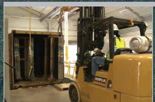
Forklift dragging a bundle out of a closed-top container
