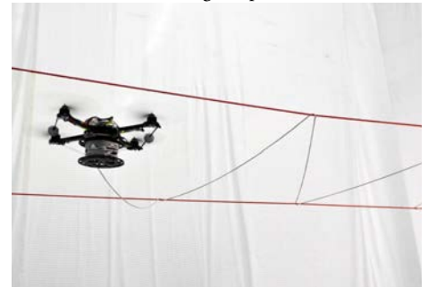
Researchers at ETH Zurich are investigating how drones could be used to build tensile structures (Photo: Professorship for Architecture and Digital Fabrication, ETH Zurich and Institute for Dynamic Systems and Control, ETH Zurich)
