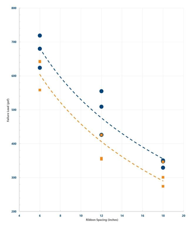
Relationship between measured failure loads and adhesive spacing for Polymer coated Glass (Type A-blue color) and Cellulosic Felt (Type B-yellow color) facers.
