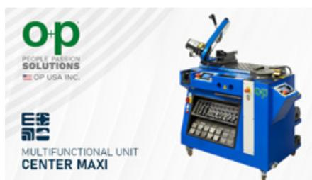
CENTER MAXI is the **O+P's** multifunctional unit for hydraulic rigid tubes' complete assembly. This mobile center allows many operations such as cutting, internal and external deburring, bending, pre-assembling rings according to DIN 2353 standards, 37° flaring of rigid stainless steel (AISI 316 TI) and carbon steel (ST 37.4) rigid tubes, from 6 to 42 mm and 4 mm thick fittings complying with SAE and JIC standards. One of the main
