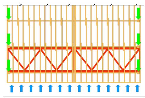
it is assumed that the posts (to which the truss will be attached) do not transfer shear, but do help prevent truss chord buckling. To determine shear wall truss component forces, model the truss as an independent component, with the shear force applied along the top of the truss, and the bottom/base of each chord pinned to a support. Each resulting support reaction is equivalent to the minimum total force that must be transferred from the truss chord into the
