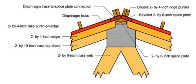
Cross-sections through diaphragm trusses (red elements) shown in figures 2, 5 and 6. Lumber sizes are nominal.
