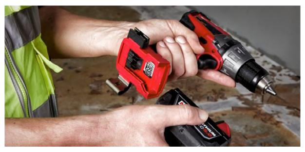
Milwaukee One-Key Tools connect through Bluetooth to an inventory management app, and other assets can be included in inventory through QR Codes or by using a Bluetooth-enabled TICK button.
