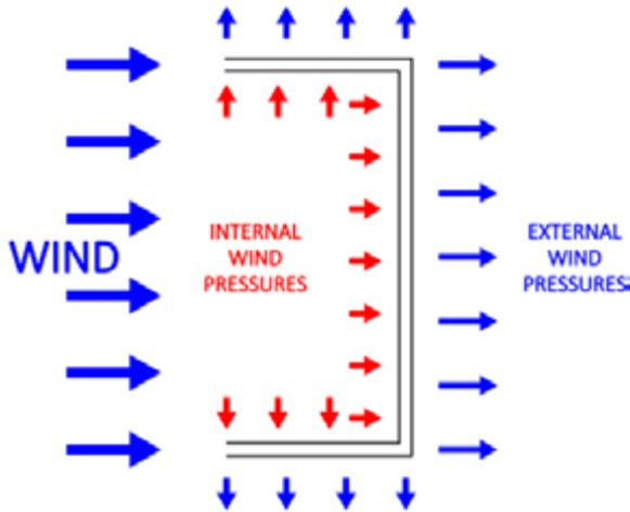
Figure 3 Plan View of a Partially Enclosed Building showing internal pressurization<sup>35</sup>
