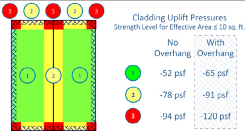
Negative (uplift) pressures are much higher at edges and corners of gable roofs, especially above overhangs. [Graphic and figures courtesy of Halberg Engineering, based upon  $q_s = 26$  psf and using ASCE 7-16, Figure 30.3-2B]
