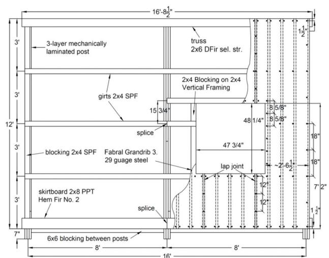
Figure 2. Case 2: 4' x 4' window opening with extra fasteners around the window
