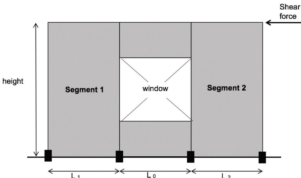
**Figure 6.** Sketch of the segmented shear-wall approach. Locations of hold-downs are marked.
