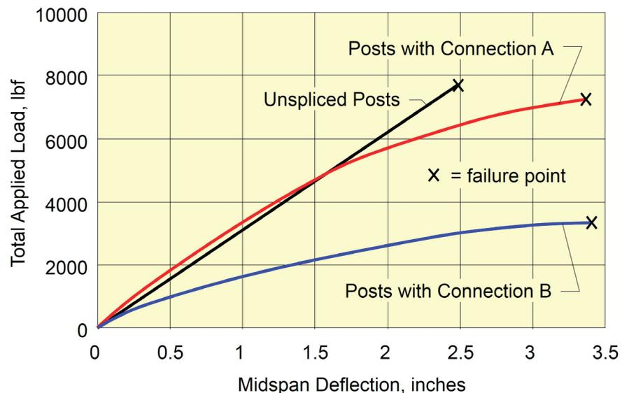
**FIGURE 8.** Results of bending tests showing the impact of cutting posts and splicing them back together with two different mechanical connections
