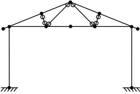
**FIGURE 2.** Circles on the ends of the web members indicate that the end is pin connected to the chords.
