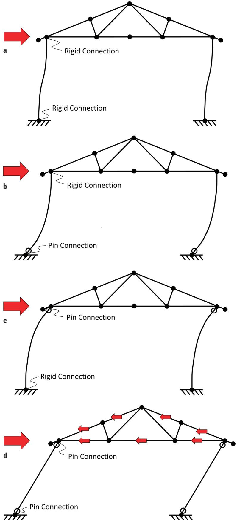
**FIGURE 3.** Influence of post end fixity on the racking resistance of a primary frame. A rigid-rigid combination (a) is four times stiffer than a rigid-pin connection (b) or a pin-rigid connection (c). The pin-pin combination (d) results in an unstable situation unless diaphragms resist sidesway.
