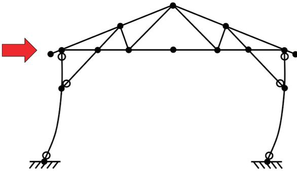
**FIGURE 4.** Use of knee braces to resist sideways when posts are pin connected to truss and concrete base
