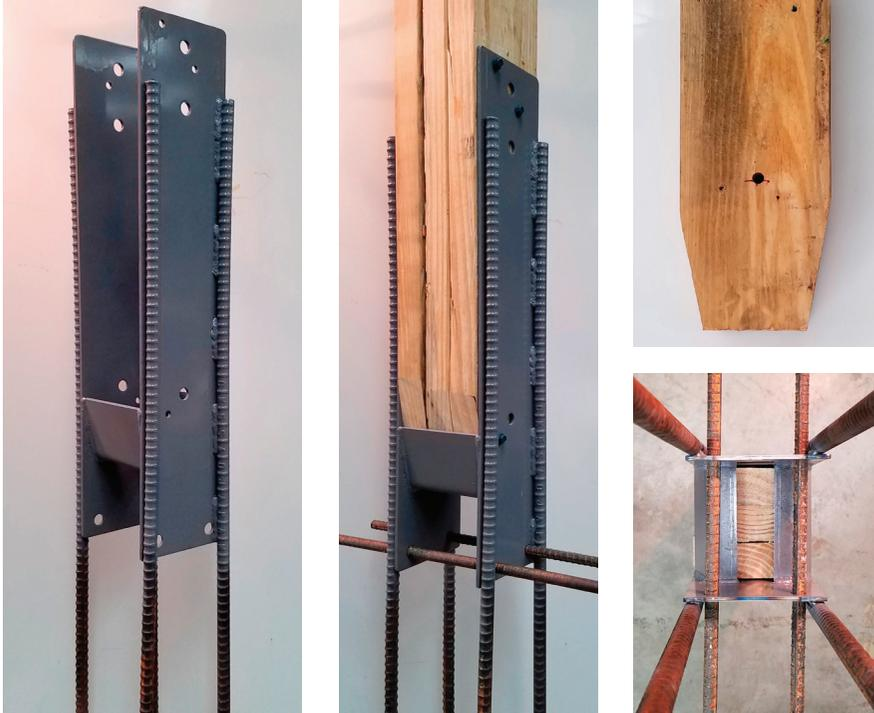
**FIGURE 12.** Recommended 2016 UW-Madison wood post-to-concrete connection design without wood post (*left*) and with wood post (*center*). The tapered wood post end (*upper right*) and a view from the bottom showing space between shoe angles (*lower right*) are shown.
