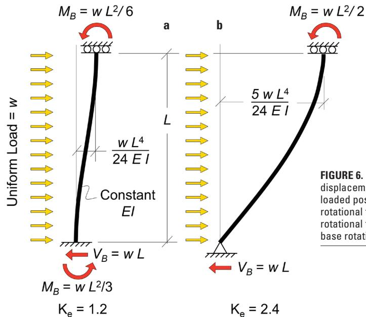
**FIGURE 6.** Forces and displacement for uniformly loaded posts with top rotational fixity and (a) base rotational fixity, and (b) no base rotational fixity (right)
