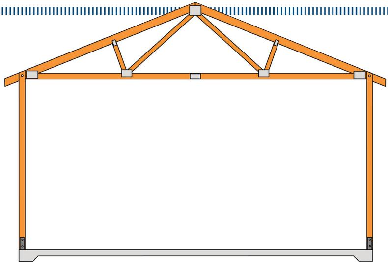
**FIGURE 1.** Primary frame of a post-frame building (*top*) and corresponding structural analog (*bottom*).
