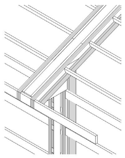
Figure 4 Closeup of purlin and grit termination.
