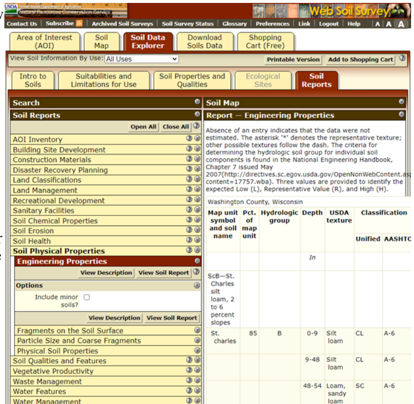
Figure 1: Partial soil report showing engineering properties obtained from the USDA/NRCS Web Soil Survey online app.
