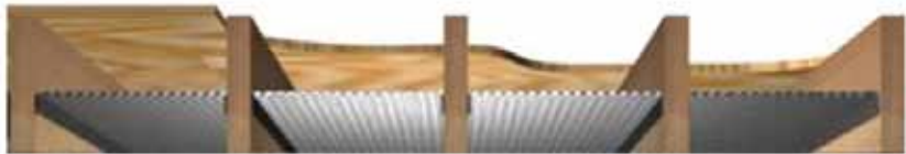
Figure 3. Reflective insulation installed in floor and wall applications
