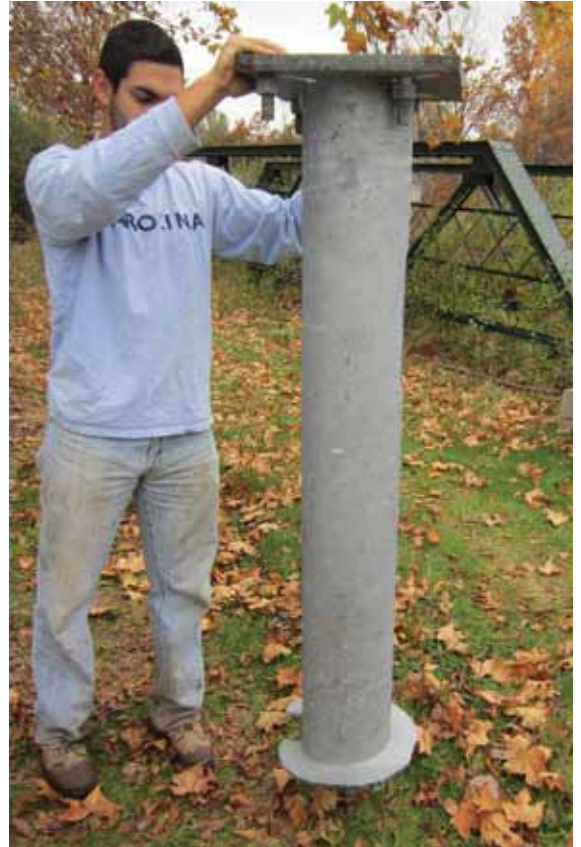
Figure 1. Typical screw-pile foundation used for post-frame buildings
