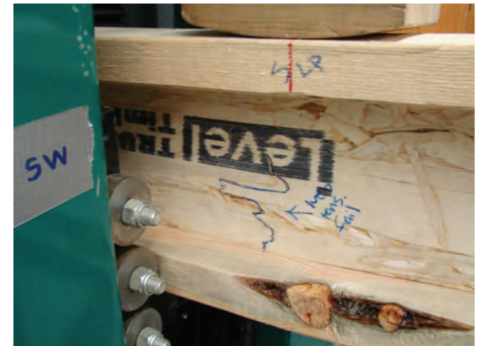
Figure 9. Typical I-S failure of the web in flexure (fracture identified by blue line below load block).
