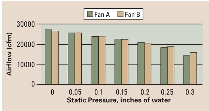
Figure 2. Airflow performance for two brands of 48-inch, belt drive ventilation fans with as installed accessories in place.
