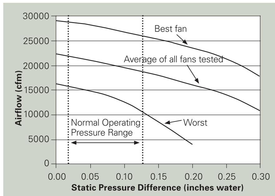
Figure 1. Airflow delivery for the best and worst 48-inch fans with 1 hp motors (BESS lab test data)
