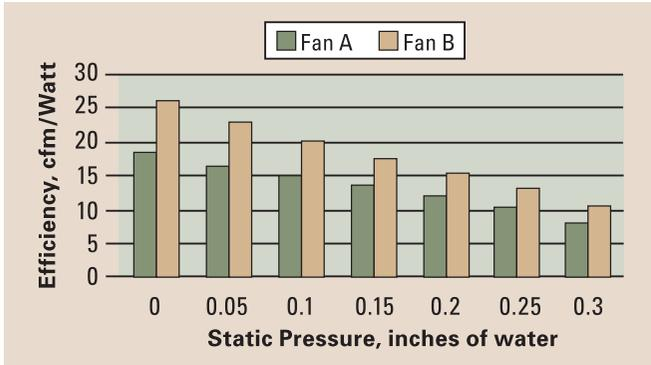
Figure 3. Fan efficiency for two brands of 48-inch, belt drive ventilation fans
