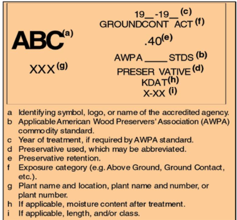
Figure 1. Typical quality mark for preservative treated lumber to conform to the ALSC accreditation program.
