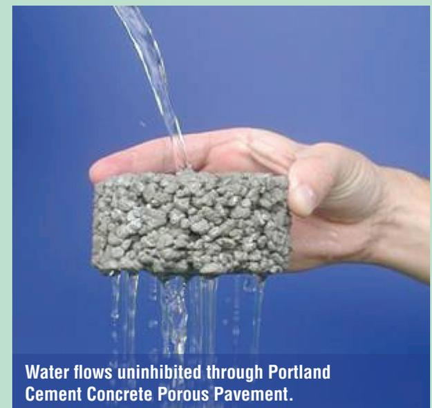
Water flows uninhibited through Portland Cement Concrete Porous Pavement.
