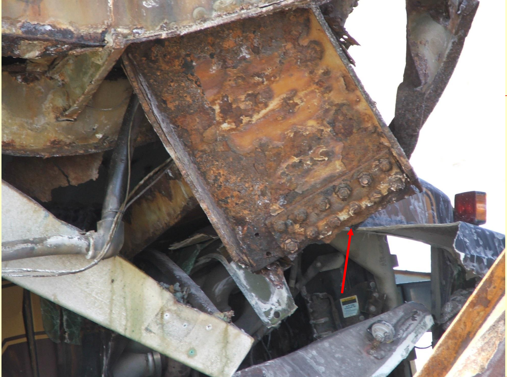
Failed shear tab “A” only 10% effective area remaining
