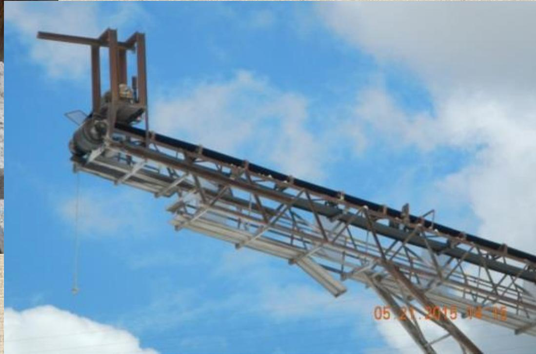
Near Miss - May, 2015 at a sand & gravel mine - An inspection party walked up the wood plank walkway to inspect the conveyor head pulley. As they started back down a section of the walkway unexpectedly dropped out from beneath the MSHA inspector leading the party. He escaped the 30 foot fall to the ground by holding onto the
