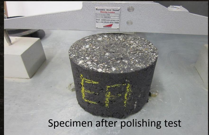
Specimen after polishing test
