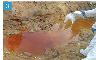
3 ... to turn bright red: oxidation is underway Time: 10 secs after application
