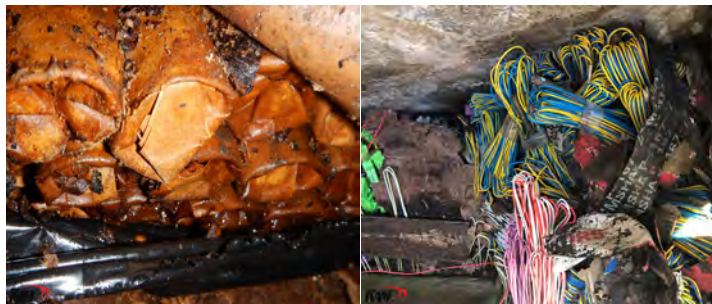
ABANDONED DYNAMITE & DENONATORS
