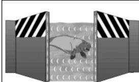
from state-of-the-art piezoelectric composite transducer elements that operate as both transmitters and receivers. Transmitter units, vertically spaced about six inches apart along one gate, emit narrow high frequency acoustic beams
