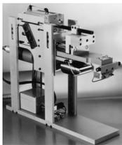
Wilmington, MA...Stapla Ultrasonics is introducing its new K1 Plastic Tube Sealer to hermetically end-seal thermoplastic and laminate tubes. The system incorporates advanced technology originally developed for Stapla's K1 high precision ultrasonic plastic welder for automotive, appliance, medical, and electronic applications. Using this new technology, the K1 Plastic Tube Sealer produces clean, high quality, wrinkle-free seals.
