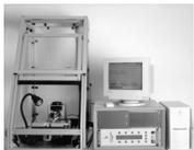
Wilmington, MA...Stapla Ultrasonics' new Ultraindexer system is designed to accurately and automatically weld multiple connections or terminals to Flexible Flat Cable (FFC) as thin as 0.002" and other components.
