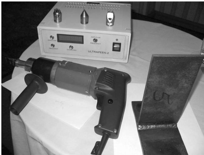
*Hands-on demonstration of ultrasonic peening of welds in steel plate.*
