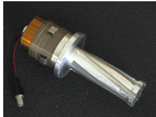
Figure 4. Solid model and photograph of finished transducer for hammering and rotating a work piece. (L.N. Domm, Y. Bar-Cohen, S. Sherrit, JPL USRP student final report, http://usrp.usra.edu/technicalPapers/jpl/DommMay11.pdf ). Courtesy of JPL/Caltech/NASA
