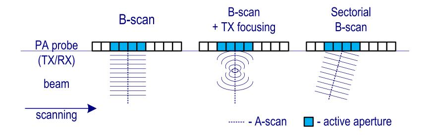
B-scan / Beamforming method:
