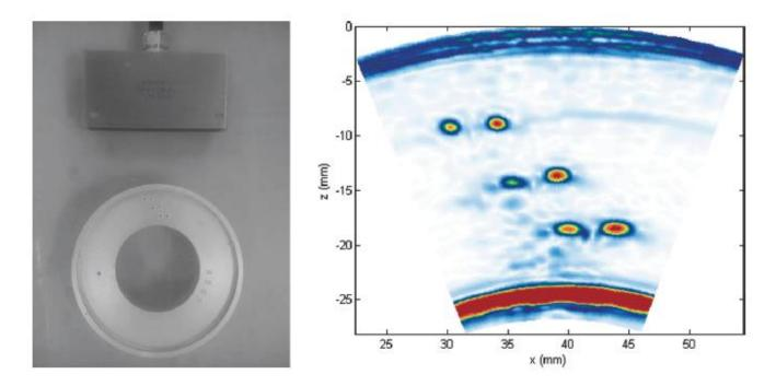
Aluminum ring with 3 pairs of SDH
