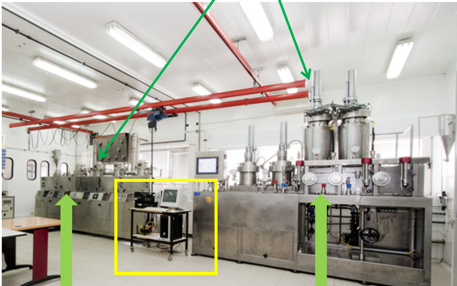
Pilot Plant PFS20 5 L Extractor Unit 1 Basket/Extractor
