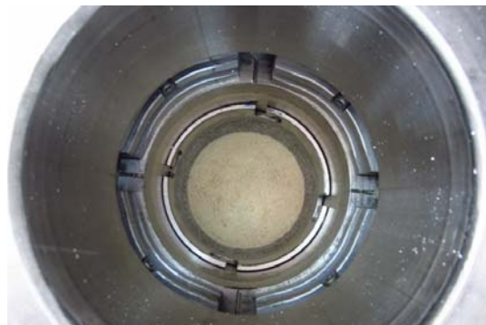
Top view of the extractor with 1,5 kg of grounded almond in the basket
