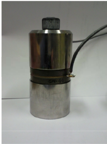
Ultrasonic Piezoelectric Transducer – Langevin Type
