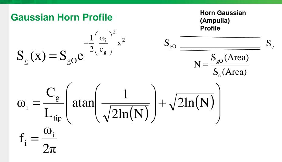
After Kleesattel, where  $\omega$  is angular frequency, C<sub>g</sub> is the acoustic velocity, L<sub>tip</sub> is the length of the tip, and f<sub>i</sub> is the resonant frequency
