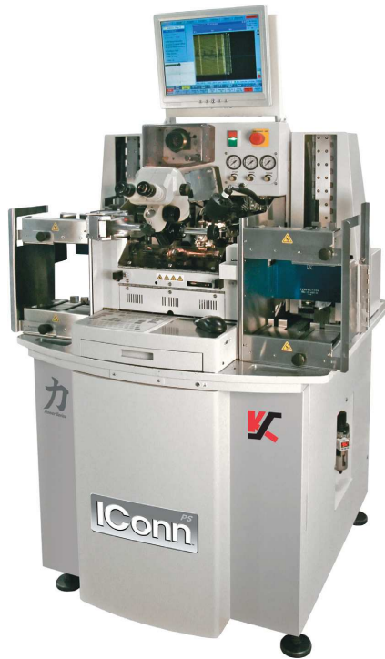
Kulicke & Soffa's Flagship Semiconductor Wire Bonding Machine
