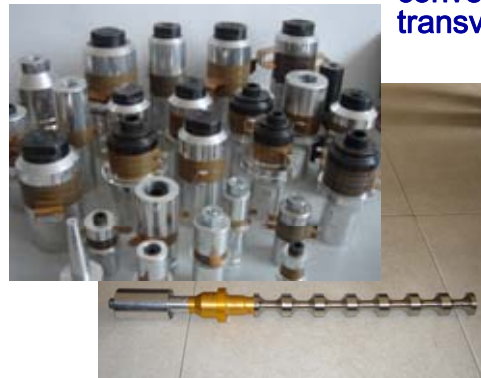
Sonochemistry transducers and the increased radiation surface
