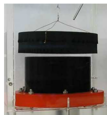
Total acoustic output total of a HITU-transducer measured up to a power level of 420 W using a radiation force balance set-up.
