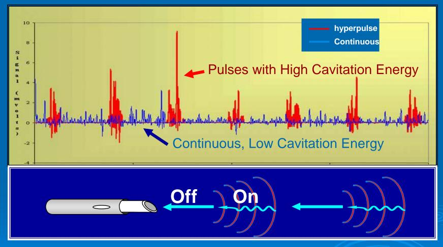
More cavitation (cutting) energy delivered with pulses than with continuous ultrasound at same power (stroke).
