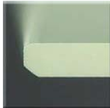
Cut surface of tantalite acid lithium thickness 0.4 mm
