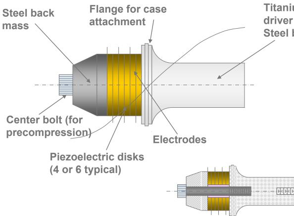
Titanium or aluminum front driver (front mass). Ti/Al front, Steel back provides boost
