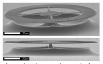
A scanning electron micrograph of a microdisk similar to the one researchers used to create their new ultrasound sensor.
