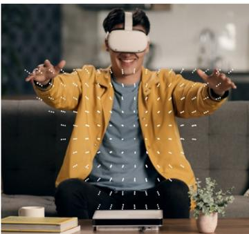
*The Emerge Wave-I device uses ultrasonic waves to create the sensation of physical touch in the metaverse.*
