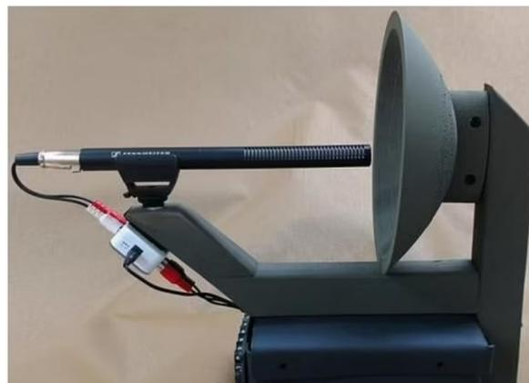
*The handheld Acoustic Hailing And Disruption (AHAD) system records a subject's voice then amplifies it and plays it back on a slight delay, perhaps a few hundred milliseconds. "Due to the delayed auditory feedback effect, the target speaker's concentration will be disrupted," reads the device's patent application, which was approved.*
