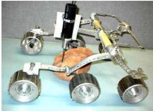
Simple feasibility tests was made operating the USDC from the Sojourner frame.
