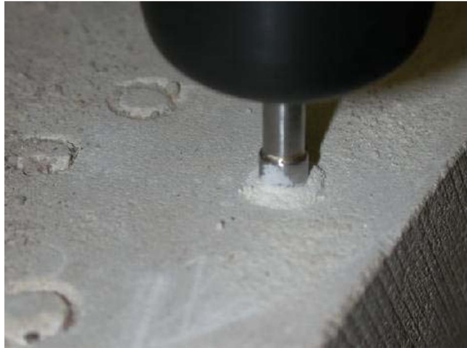
The sampler in action drilling limestone and accumulating powdered cuttings inside the bit
