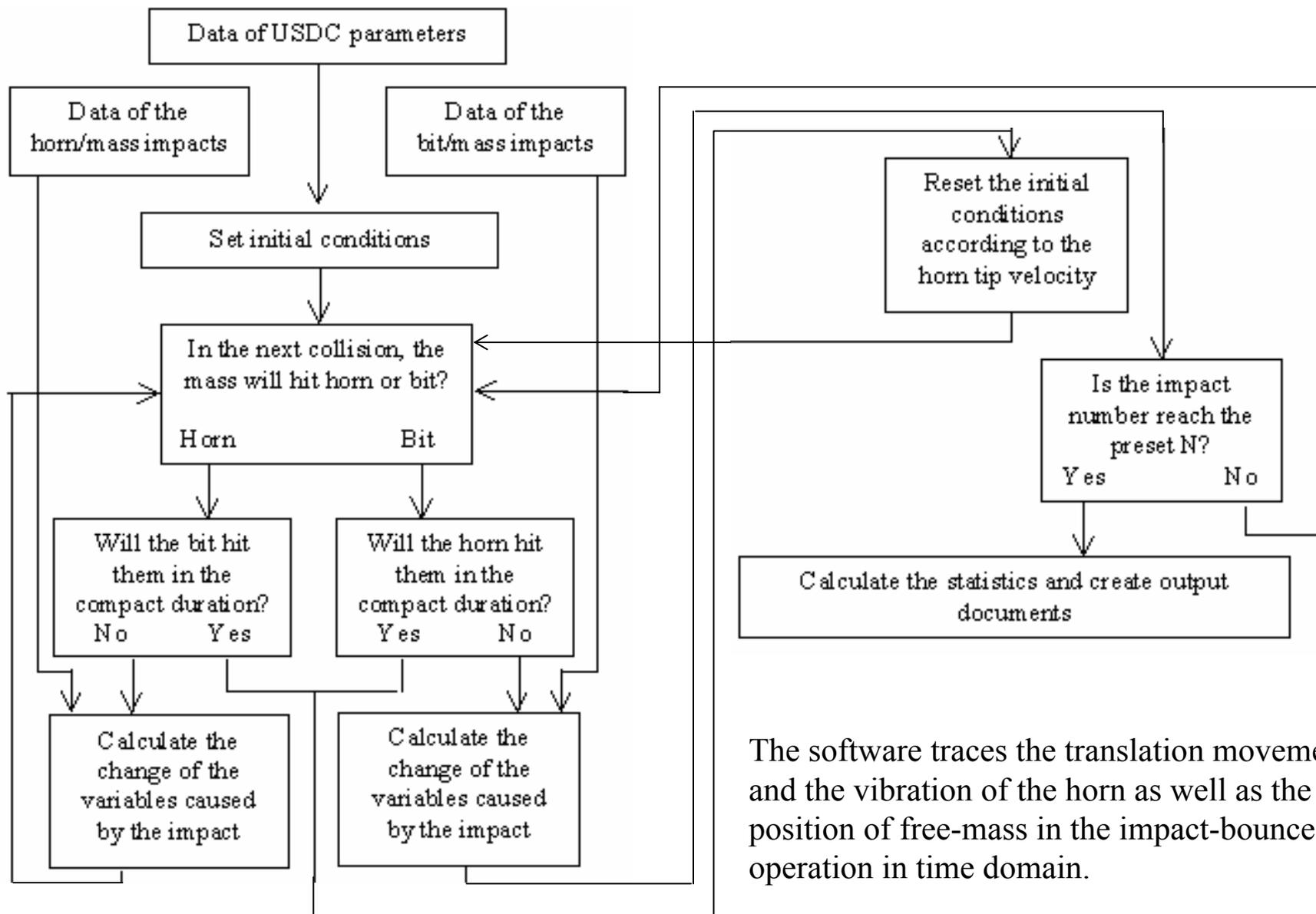
The software traces the translation movement and the vibration of the horn as well as the position of free-mass in the impact-bounce operation in time domain.
