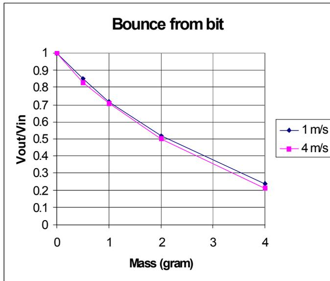
FEM results of the free-mass bounce from the drill bit. The free-mass is 2 grams and the incoming speed is 1 m/s. The rebound speed is 0.53 m/s and contact time 16  $\mu$ s.
