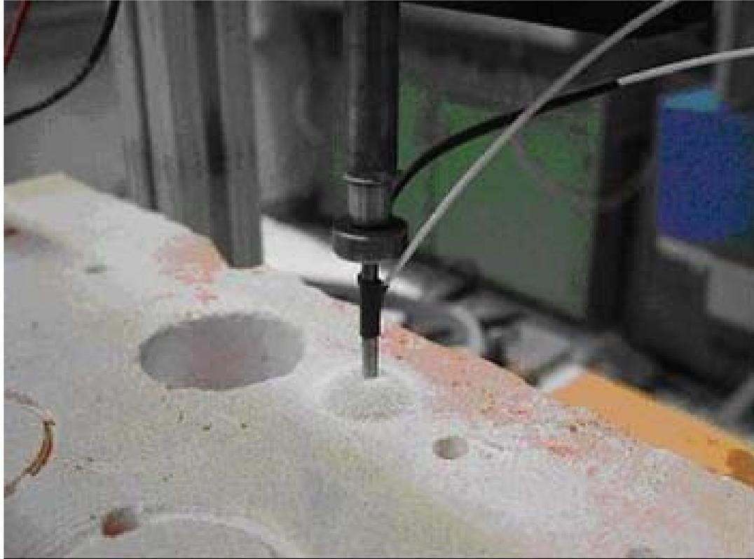
Drilled 1.1-inch deep hole on limestone, no damage integrated fiber optic was found.
