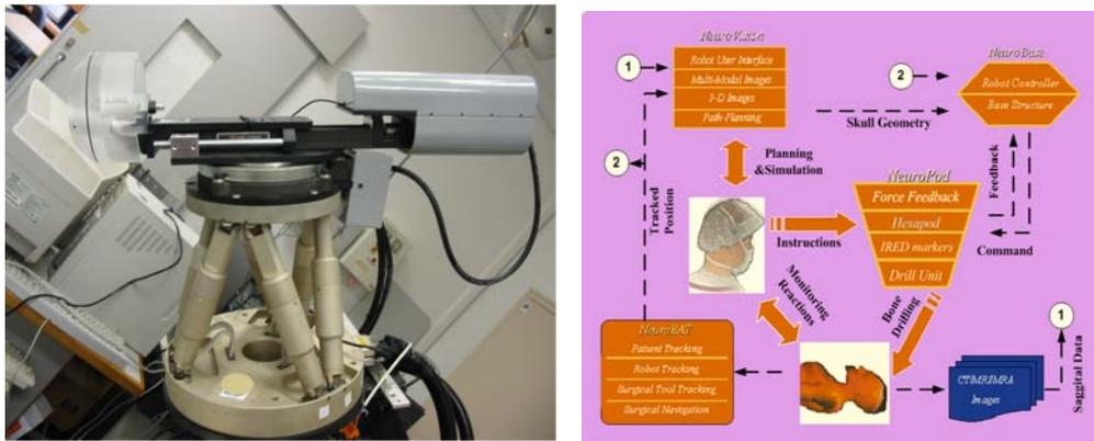
Figure 3: The Neurobot base mounted with a HIFU-effector (a), various modules of Neurobot (b).
