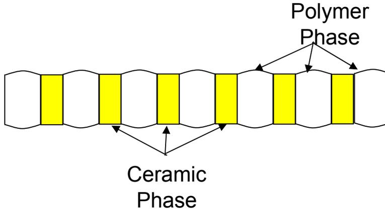
Active materials and binding polymer have different mechanical properties and hardness, commonly causing unevenness at the boundaries between the two materials after grinding of composites.
