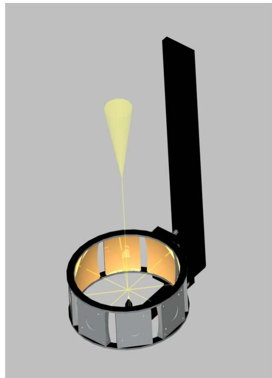
Figure 1. Schematic Diagram of HIFU Hydrophone Concept.
